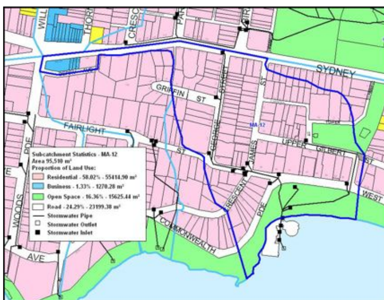
Figure 5.12.12 - Map of land use and stormwater system for Sub-catchment MA-12, Manly Cove
