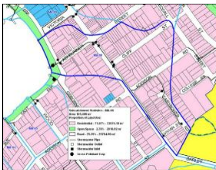
Figure 5.12.8 - Map of land use and stormwater system for Sub-catchment MA-08, Manly Cove
