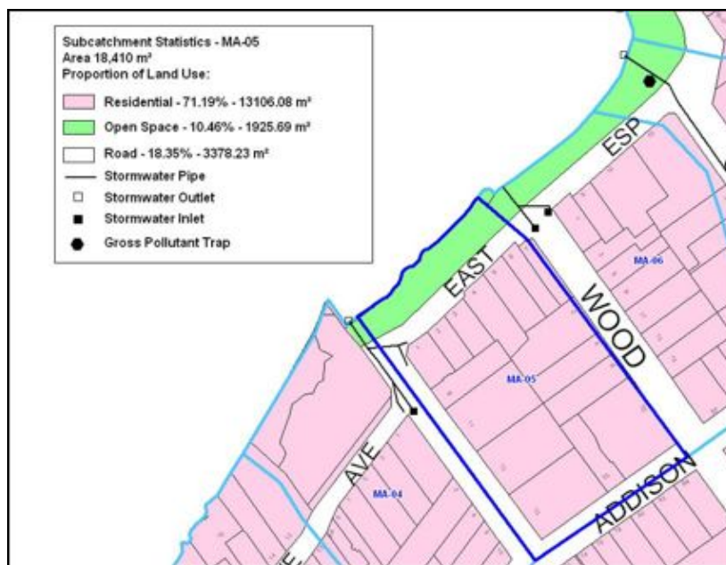
Figure 5.12.5 - Map of land use and stormwater system for Sub-catchment MA-05, Manly Cove
