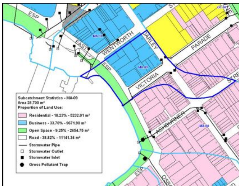
Figure 5.12.9 - Map of land use and stormwater system for Sub-catchment MA-09, Manly Cove
