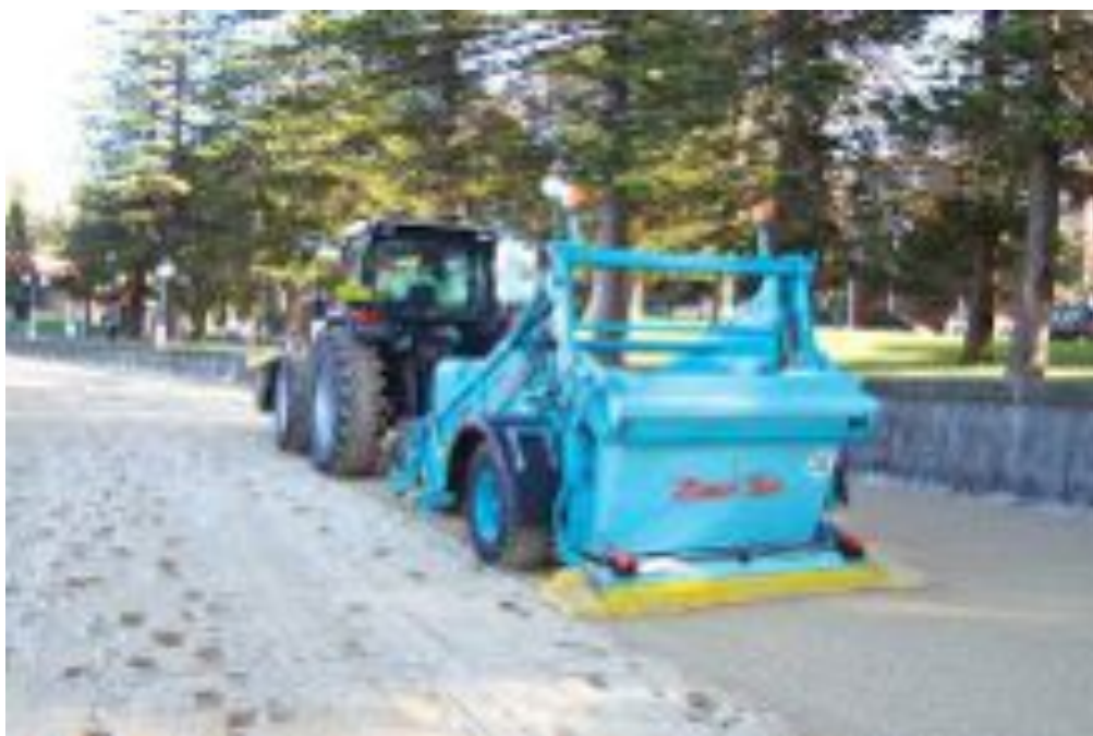
Figure 8.4.1b - BeachTech 2000 rake/sieve used to clean litter and debris off Manly Cove beaches
