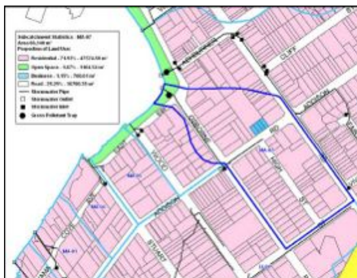
Figure 5.12.7 - Map of land use and stormwater system for Sub-catchment MA-07, Manly Cove
